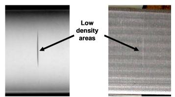
Figure 2. X-ray (on left) showing an apparent void and the cross section of warhead (on right) showing no discontinuity.
