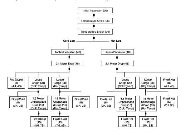
Figure 5. Testing sequence for the extreme environmental conditioning of PAX-3 loaded BDM warheads.
