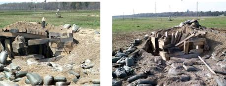
Figure 3. Bunkers tested with standard AI Comp A3 warheads (on left) verses PAX-3 tested bunkers (on right) showing more damage.
