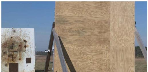
Figure 4. Surrogate target used to initiate BDM warheads in delay mode with steel back backstop.
